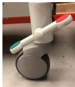
Wheel Lever GREEN Down Directional Steering castor engaged at rear of couch
